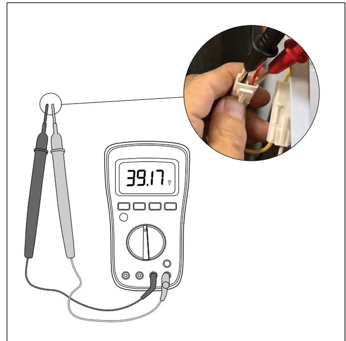
Figure 8 Applied Voltage Measurement Method
