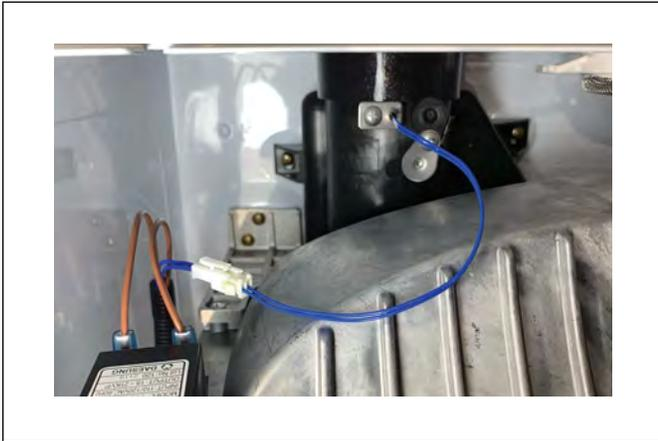
Figure 61 Exhaust Temp. Sensor
