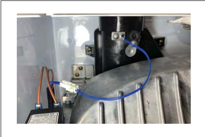
Figure 67 Exhaust Temp. Sensor
